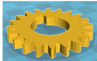
Fig. 8. 3D representation of the toothed gear to be manufactured with the printer
