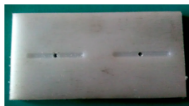
Fig. 11 Guide element with greasing channels manufactured with the engraving machine
